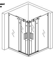
6. Apply silicons seelend to all joints between fixed glass panel, wall profile and enti-water strip on the base. Don't use the enclosure for 24 hours, to allow the slicons to dry completely.
