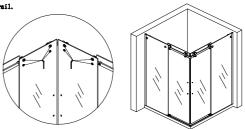
$\delta_1$  Put the F-rubber on the fixed panel and 90  $^{\circ}$  magnetic stripe insert the door and fix the handles.
